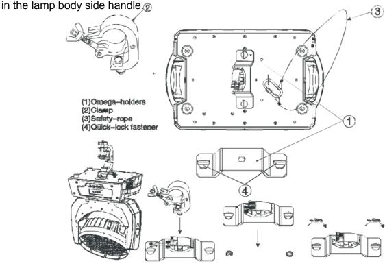
Warning: Do not use the hand of the LED moving head to up and down or fix.
